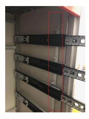
Once correct operation of the locking bar is manually confirmed check by inserting the key and operating the lock function. The bar will move up and down as the key is turned when operating correctly.
