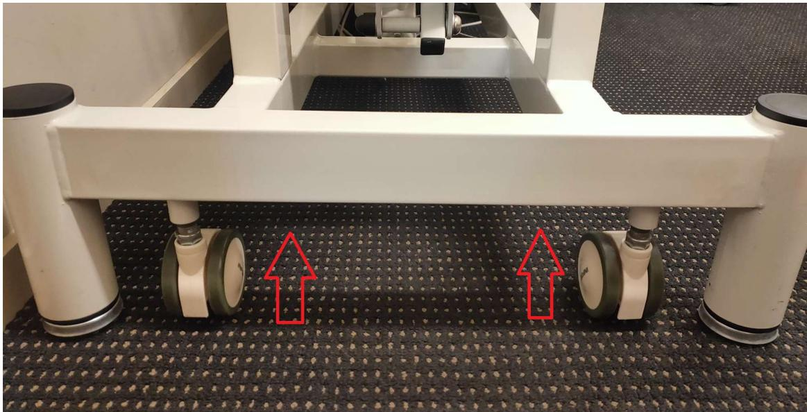
The next step is to pull the locking lever up and down quick approx. 5 times. Then push the lever back down to lock the wheels. This will re-engage the wheel system.
